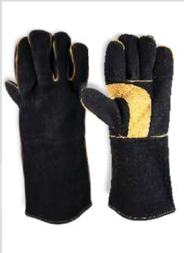
9739-W19-GW Selective black split leather with Reinforced yellow palm for Added durability Withstand high temperature Wing thumb continues with one piece back Full fleece liner & denim cuff with piping Size 16" for forearm protection
