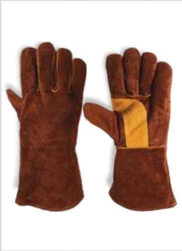
9721-W17-BW Selective cowhide brown split leather Reinforced yellow palm for Added durability Withstand high temperature Wing thumb continues with one piece back Full fleece liner & denim cuff with piping Size 16" for forearm protection
