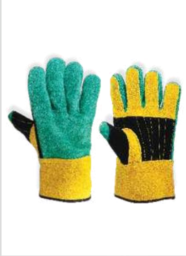
9717-W12-YW Cow split leather heavy duty gloves For steel and metal handlings Four layers leather protection One layer kevler protection Zipper are stitched under all fingers Size 10 inch
